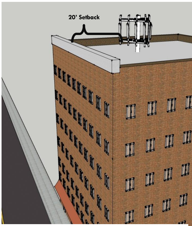
Figure 15.14.130-3 Rooftop towers and antennas shall be camouflaging shall be set back a minimum of if located within 20' from of the roof's edge.
