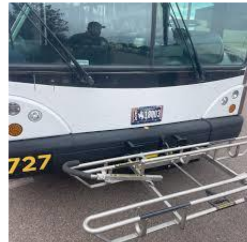
Figure 32: Bicycle Racks on UWYO bus.
