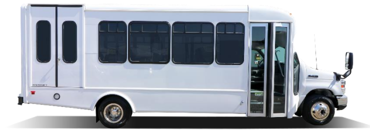
Figure 26: Example 25' high-floor bus.
