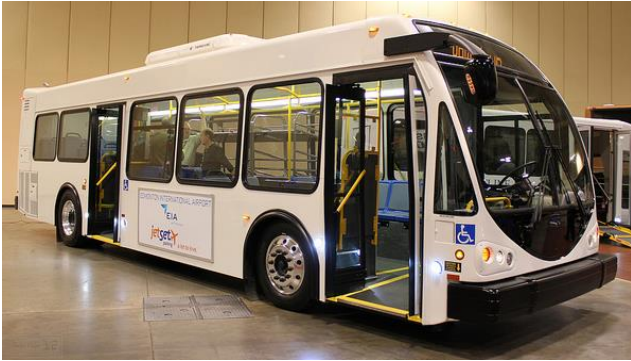
Figure 25: Example 30' low-floor transit bus.
